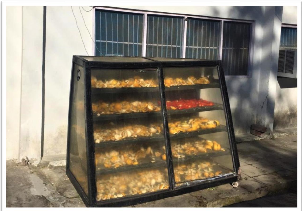
Image of a Solar Dryer (cold).
